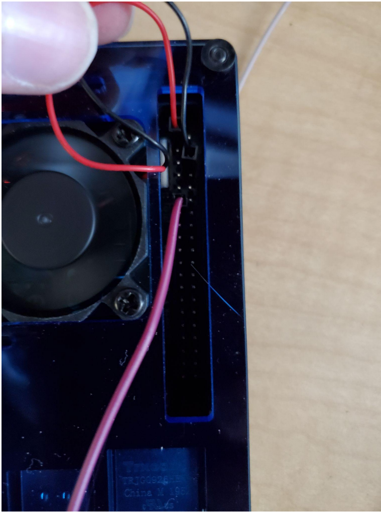
Figure 12: Proper connection pin for camera arm servo control wire.
